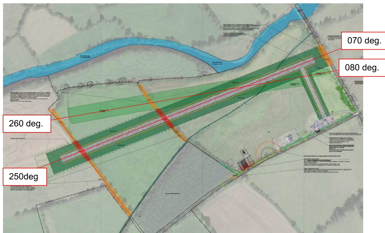
Figure 10-10-7: Showing the proposed runway heading change of -10^\circ between the existing and proposed arrangement at the Rathcoole Aerodrome (Cathal O'Meara Landscape Architects, 16/06/2025).
